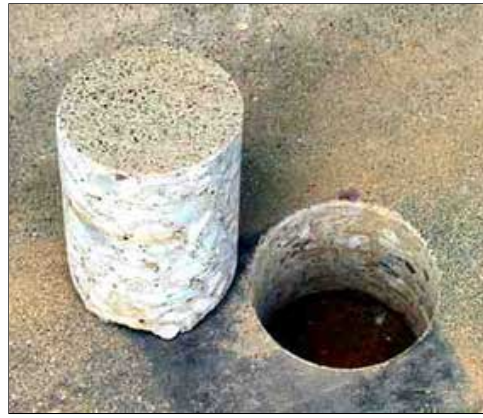
4-IN CORE DRILLED IN CONCRETE PAYMENT
